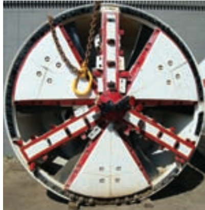
Figure 1: TBM with flood doors
