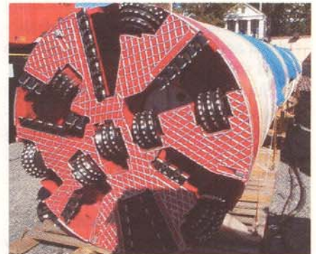
Figure 5: Contract Specified MTBM to Excavate Till with Boulders
