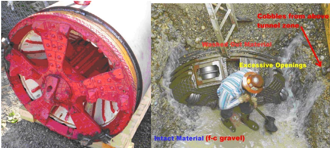
Figure 8: Bad Judgment in the Selection of Cutterhead for Indicated Conditions
